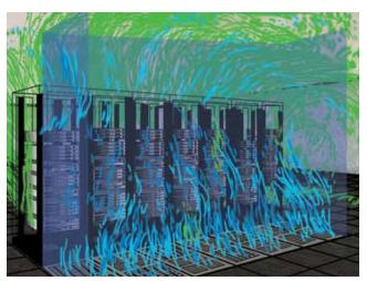
The above CFD modeling illustration is of efficient data center air flow due to perforated tile placement and aisle containment.
